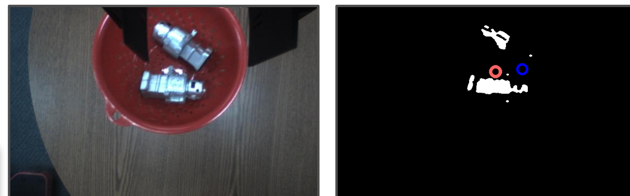
Fig. E - On the left is an image taken from Baxter's hand camera as it hovers over a bowl of plush toy robots. To the right is the same image after thresholding is applied. The red circle indicates the center of the white pixels while the blue circle represents the center of Baxter's gripper.
