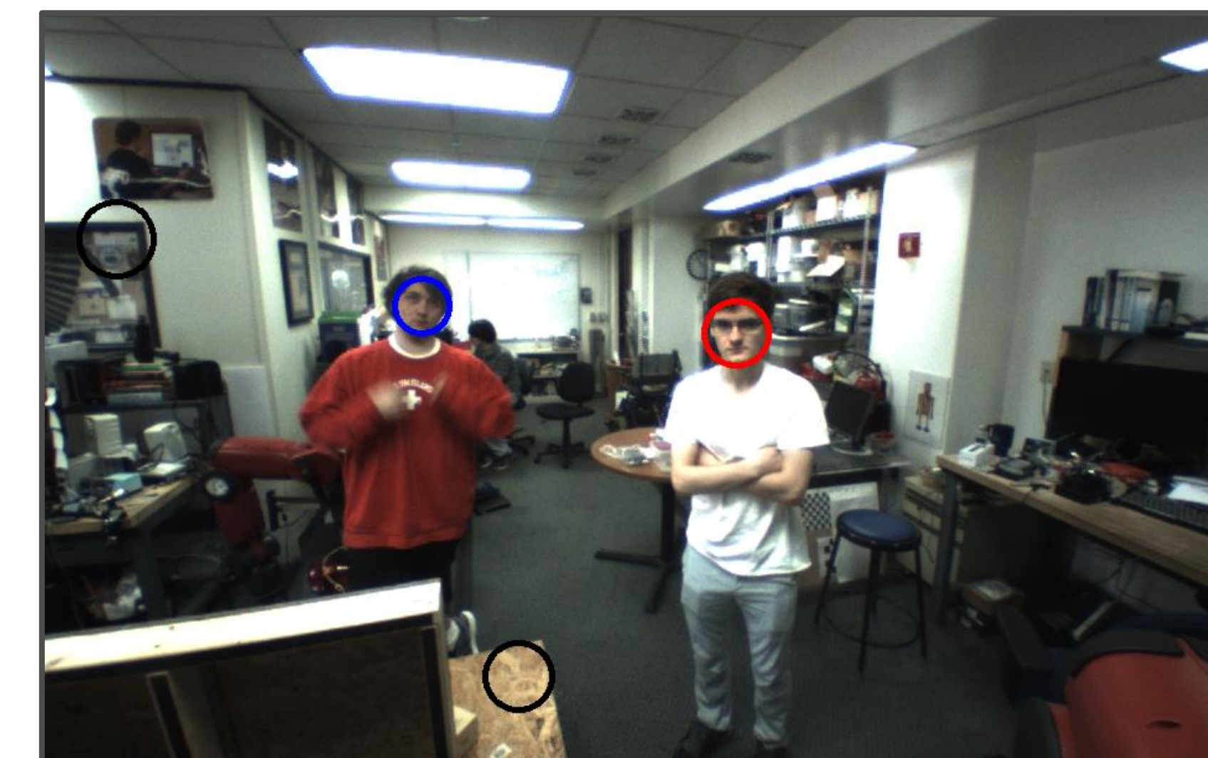
Fig. D - A view from Baxter's head camera with a face tracking overlay. A red circle is drawn around the face being tracked while blue ones are around other valid-colored faces. Black circles are placed around invalid faces.
